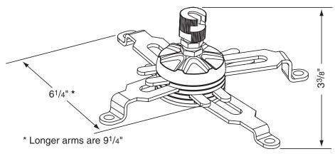
Please Note: This is total height of Universal Projector Bracket. Once attached, Universal Bracket adds a minimum of 3" to overall height.
